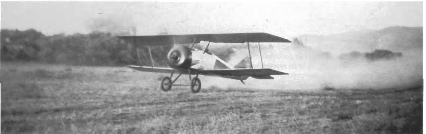
Ventura, California.—1926. Thomas-Morse S.4C "Scout" (80-hp Le Rhone 9C) taking off at Ventura Field, May 1926. Pilot is Russ Gerow's flying instructor, Air Service Reserve Lieutenant David R. Matthews, who soloed Gerow at Taft in June 1925. This image shows the clean lines of the "Scout" and evokes the typical rural setting of most airfields of the time. The Tommy's 8'7" wooden prop kicked up enough dust to make it look more "chesty" than it was, but up close the wide-open rotary must have been ear-splitting. The lack of hard shadows on the plane suggests that this photo was taken before the usual midday "burn off" of the marine layer that blankets the central California coast in spring and summer. (Photo taken by Russ Gerow) [caption continued on next page]
